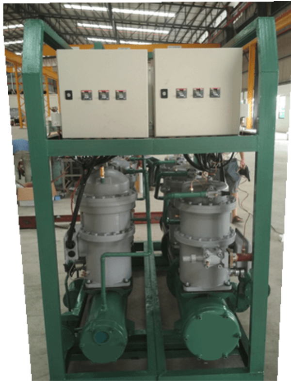
TWINS SPLIT-ABLE COMMON FRAME FOR UNITS WITH STANDBY (SEMI-HERMETIC SCROLLS)
